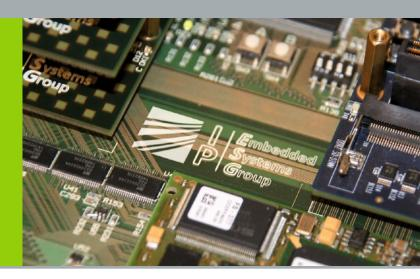
The Fraunhofer Heinrich Hertz Institute HHI offers a range of H.264/AVC compliant codecs (IPs) for use in industrial applications. Specially tailored to real-time applications, the IPs allow coding of up to 1080p resolution on current FPGA technologies. The codecs are fully hardwired implementations with low power consumption and minimal resource usage.
