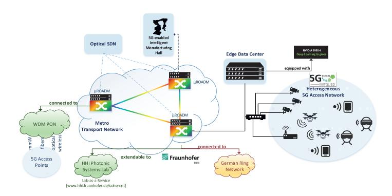
The 3-node microROADM metro network testbed hosted at Fraunhofer Heinrich Hertz Institute provides a great opportunity to perform real-field experiments including 5G-ready RAN infrastructure and edge compute capability for realizing low-latency end-to-end use-cases.
