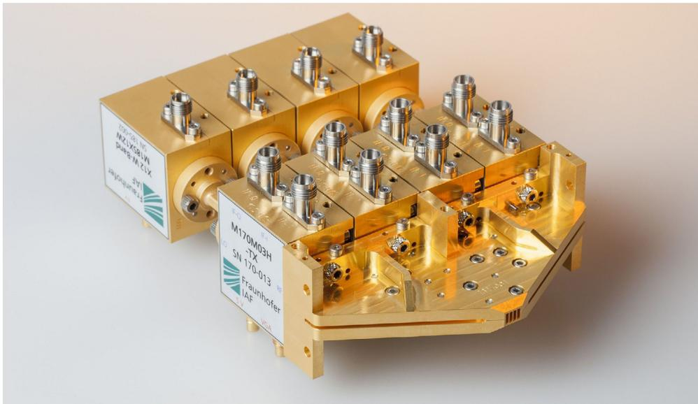
**In the TERRANOVA project, Fraunhofer IAF is focusing on the integration of wireless modules at the chip level. The image shows a functional prototype of a 300 GHz multichannel wireless system for further integration as a system-on-chip. © Fraunhofer IAF | Picture in color and printing quality: [www.fraunhofer.de/en/press](http://www.fraunhofer.de/en/press)**
