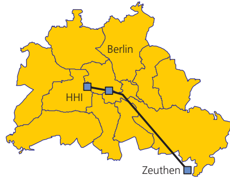
Fig. 2: Installed fibre link (77 km SSMF), which was directly connected to the test-bed at HHI
