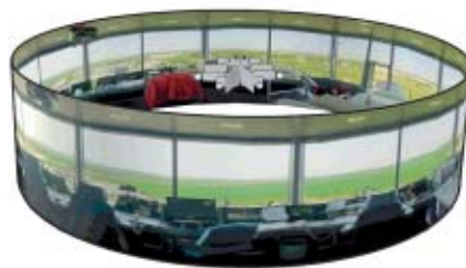
Fig. 2: 360° panorama projection with 8 XGA projectors served by two CineCard PCI boards hosted by one PC (total resolution is app. 8000 × 720 pixels)
