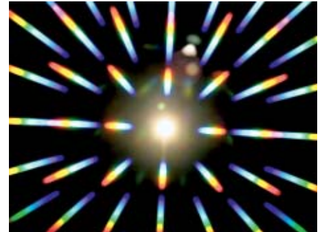
Fig. 3: A 7×7 beam splitter (see also Fig. 2) diffracts the different "colours" of white light (Halogen lamp) in various angles (negative dispersion typical for DOEs)
