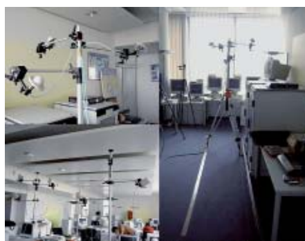
Fig. 2: Antenna configurations in mobile measurements. Left: Transmit (top) and receive (bottom) antennas. Right: The transmitter is moved on a wheeled photo stand along a 4 m track in the office.
