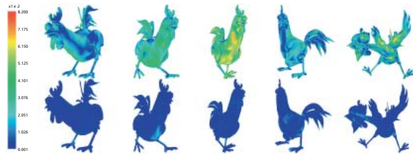
Fig. 3: Comparison of static and dynamic mesh coding at 5 different time instances: Reconstruction error using static 3DMC at 915 kBit/s (top) and dynamic D3DMC at 364 kBit/s (bottom)
