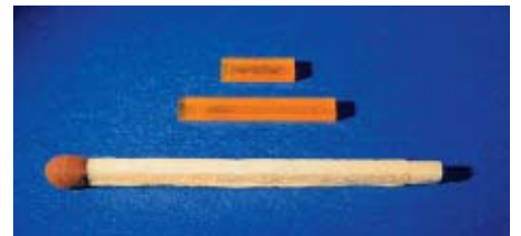
Fig. 5: Small size all-polymer components: 4-channel AWG (top), 4-channel OADM (bottom)
