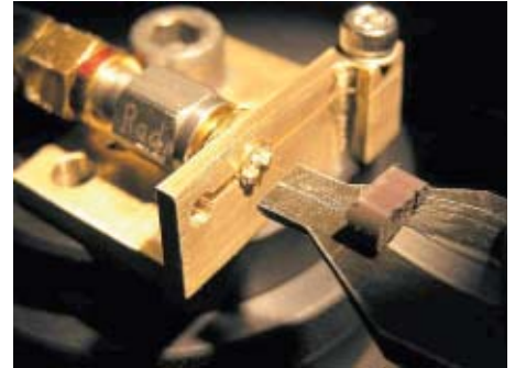
Fig. 4: Photodiode directly mounted on a V-type connector (here shown in a measurement set-up with a fibre)
