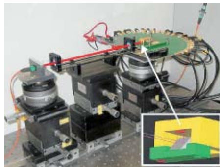
Fig. 2: Photography of the free-space optical transmission system using a 12-channel transmitter and receiver
