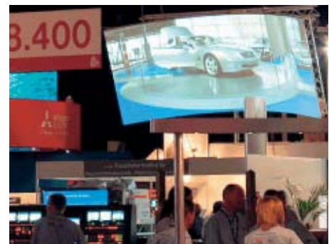
Fig. 3: Projection onto the curved surface of 72° panorama using two SXGA projectors with a total resolution of 2464 × 1024 pixels (shown at IBC 2004 in Amsterdam)
