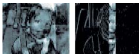
Fig. 3: Difference images between adjacent frames during a hard cut (left) and a wipe (right) used in the shot detection algorithm
