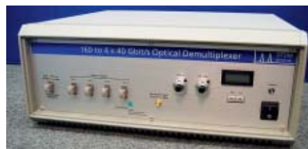
Fig. 1: One of the compact units for a 40 to 160 Gbit/s upgrade (160 → 40 Gbit/s demultiplexer)
