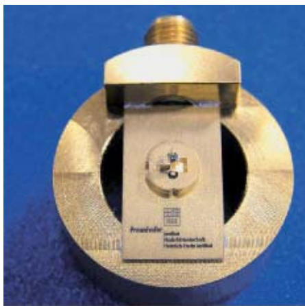
Fig. 3: Photodiode on TO-5 socket; connected by a 50 \Omega microstrip line to an SMA adaptor
