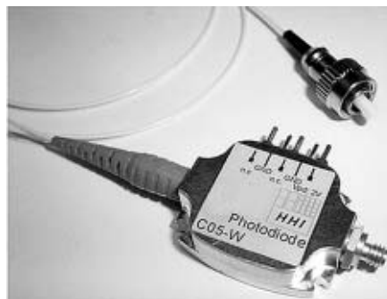
Fig. 2: Photograph of the PD module with fibre pigtail and 1 mm output connector
