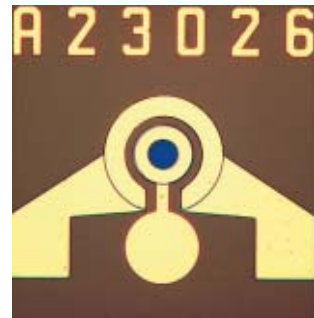
Fig. 4: Planar photodiode with RF-suitable contact pattern (ground and signal pads on front side)
