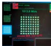
Reconstructed MIMO-OFDM data symbols from 3 transmit antennas (64 QAM)
