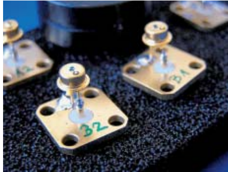
Fig. 2: TO-5 housings with laser and photodiode, connected by their 'legs' to the rear side of SMA connectors
