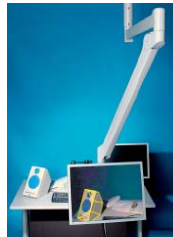
Fig. 2: The object tracker camera on top of the monitor captures the real scene. The software is recognizing the position and orientation of a known object (in this example a loudspeaker) and correctly matching the edges and a virtual texture. All processing is done in real-time. The user can freely move the articulated monitor.
