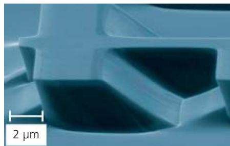
Fig. 3: Sloped sidewalls formed in InP by physical ion beam etching
