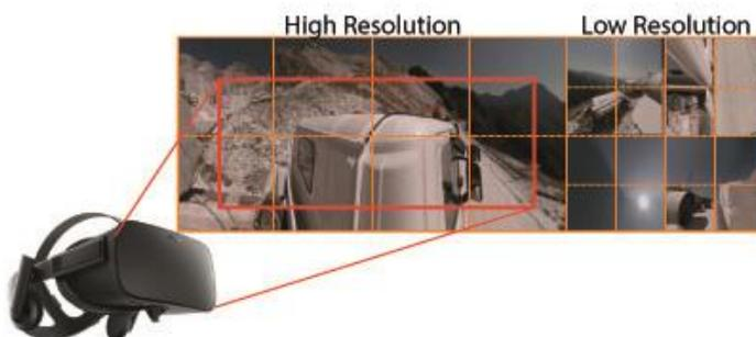
**High and low resolution HEVC tiles are mixed on-the-fly to match viewport orientation resulting in a per-user bitstream without the need for transcoding.**
