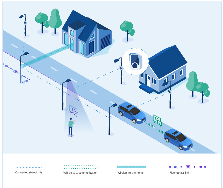
Optical Wireless link for short-range fixed access applications.
