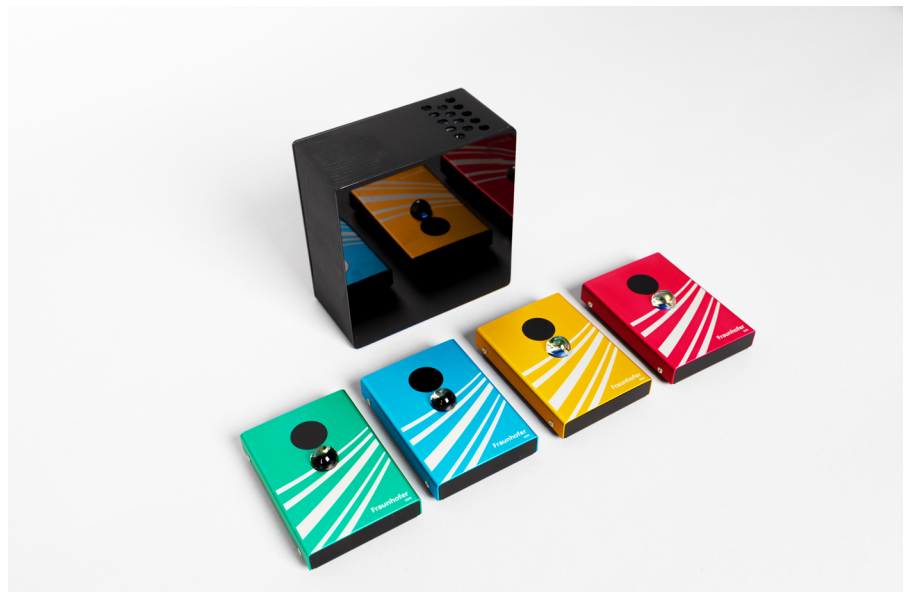
Figure 1: One or multiple LiFi antennas (black box) can be connected via powerline to the WLAN Router. With an integrated LiFi antenna and powerline profile support, which is available in the latest G.hn standard from ITU-T, multiple mobile devices can be used for robust and secure data transfer.
