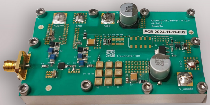
High-power TX optical frontend with 9 VCSEL arrays commonly driven by the same driver.
