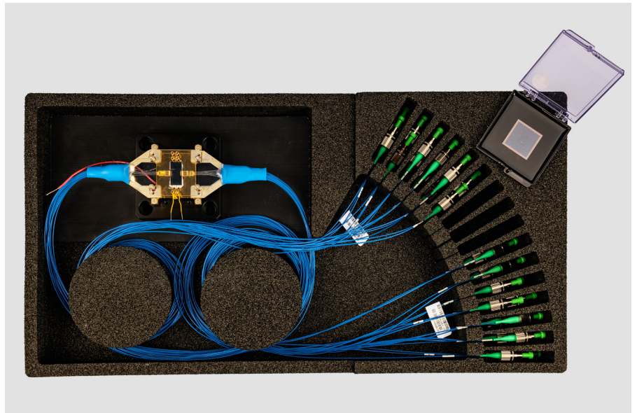
SOI-based integrated photonic reservoir hardware for smart monitoring of optical modulation formats.
