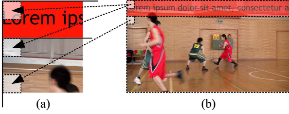
Figure 2: (a) spatially multiplexed SP and (b) associated CP with two slice segments and exemplary MVs.
