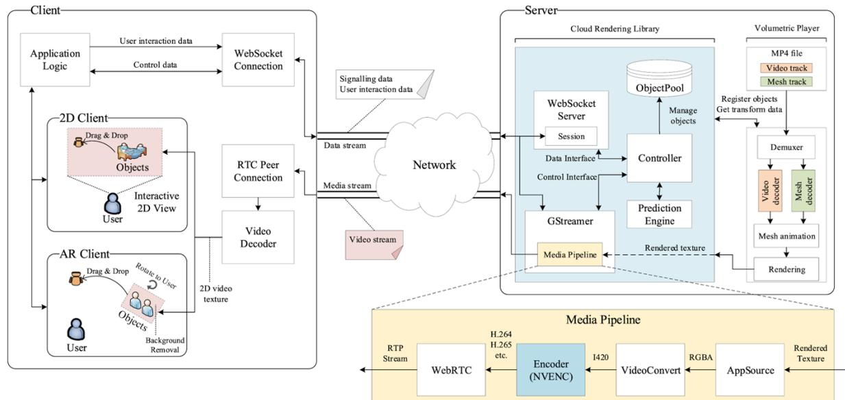
Figure 3 - Overview of cloud-based volumetric streaming framework.
