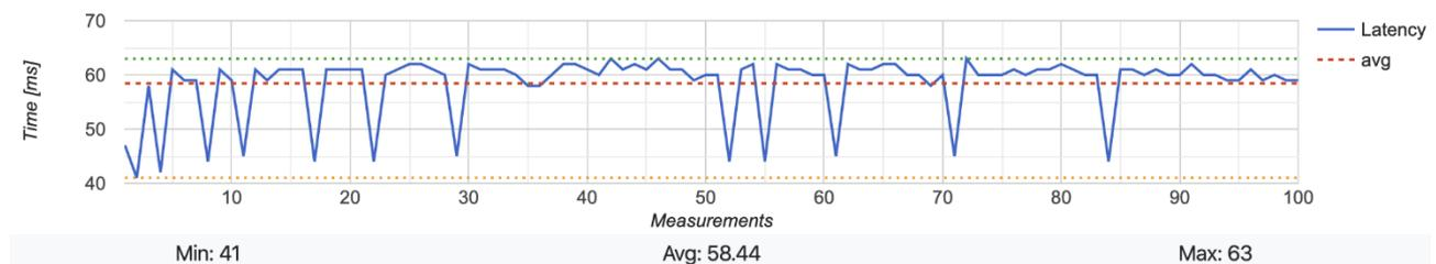
Figure 4 - Results of our motion-to-photon latency measurements.
