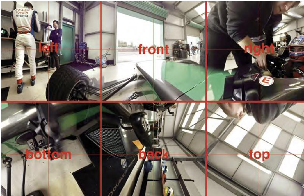
Figure 4: Segmentation of the Cubemap projection tiles
