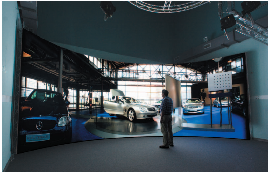
132° Panorama Projection by five SXGA+ projectors with 5000 x 1400 pixels at the HHI
