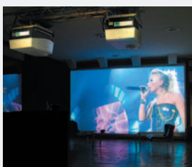
High-Resolution double projection using two synchronised beamers
