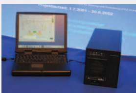
CineBox and Control Unit connected via LAN
