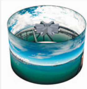
Example for an ultra high resolution 360° Panorama realized by 8 beamers
