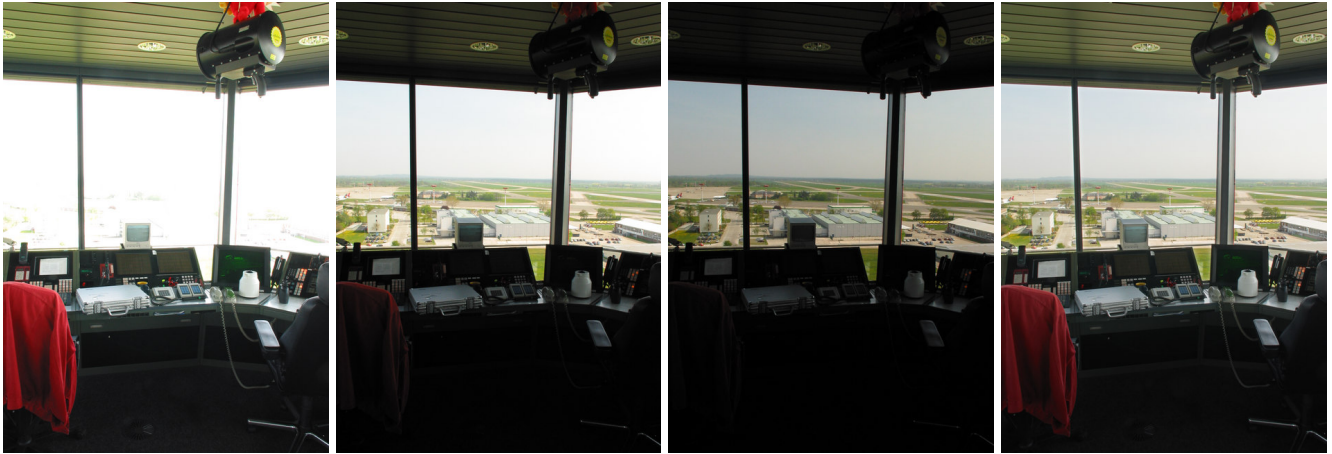
Fig. 10. Left three images: Differently exposed images from the interior of an airport tower. Right: combined image with high contrast in dark as well as bright regions.
