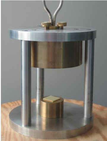
Resonator setup for material characterization.
