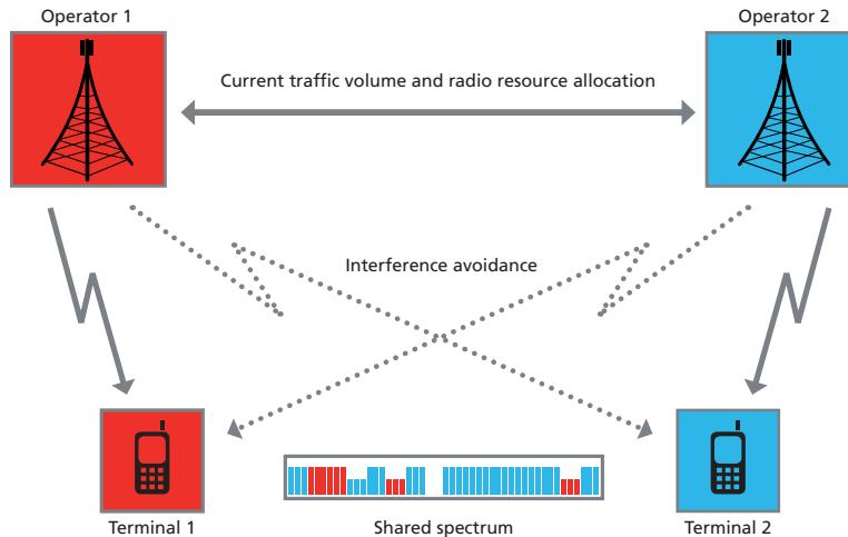
Principle of the spectrum sharing experiment explained in the text below.
